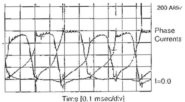
FIGURE 7: MEASURED GENERATOR PHASE CURRENTS
