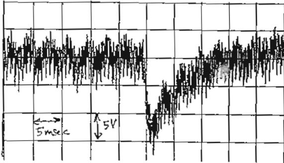
FIGURE 9: MEASURED BUS VOLTAGE DURING RESISTIVE LOAD INCREASE
