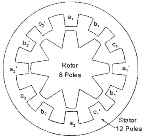
FIGURE 1: CROSS-SECTION OF SWITCHED RELUCTANCE MACHINE
