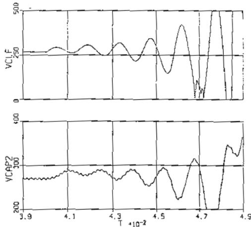
FIGURE 13: POSSIBLE UNSTABLE OPERATION PREDICTED BY COMPUTER SIMULATION
