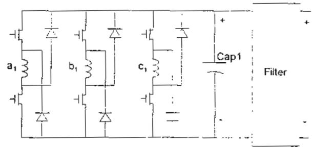
FIGURE 3: PHASE WINDING CONNECTIONS
