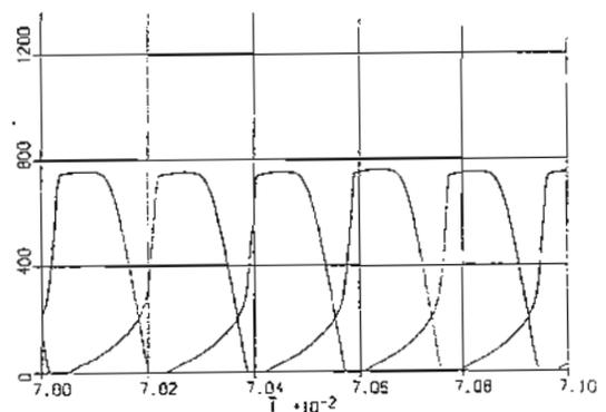
FIGURE 8: GENERATOR PHASE CURRENTS CALCULATED BY SIMULATION
