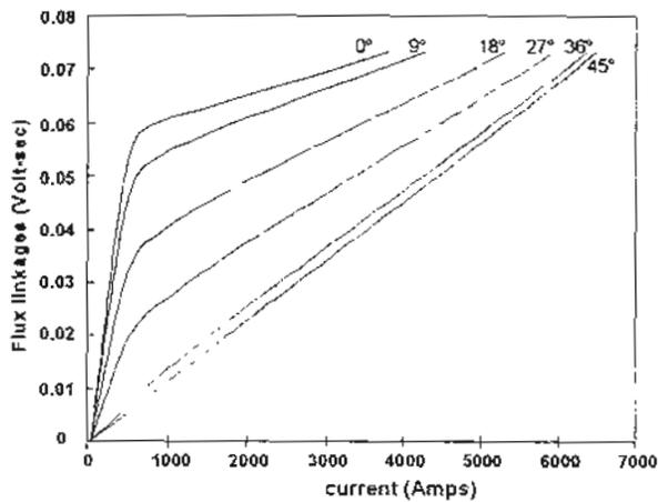
FIGURE 2: FLUX LINKAGE VS CURRENT CURVES
