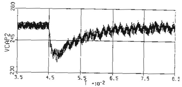
FIGURE 11: BUS VOLTAGE TRANSIENT CALCULATED WITH LARGER INTEGRATION TIME STEP
