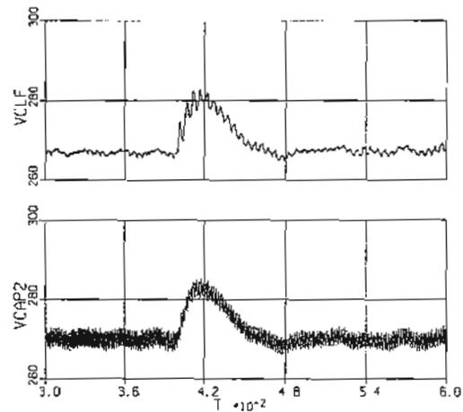
FIGURE 12: TRANSIENT VOLTAGES CALCULATED DURING CHANGE FROM RESISTIVE LOAD TO CONSTANT POWER LOAD
