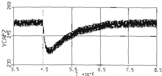
FIGURE 10: CALCULATED BUS VOLTAGE DURING RESISTIVE LOAD CHANGE
